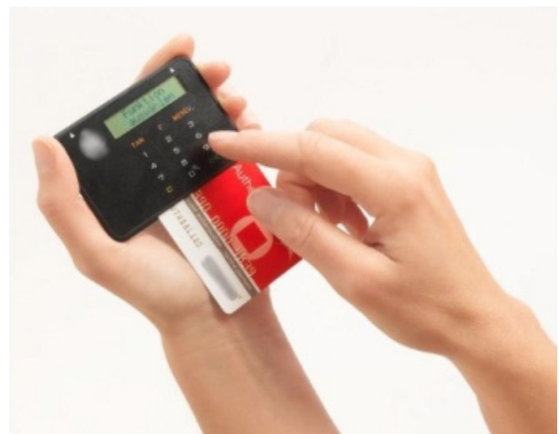
Figure 2. Strong authentication and authorization (chipTan transaction verification)
